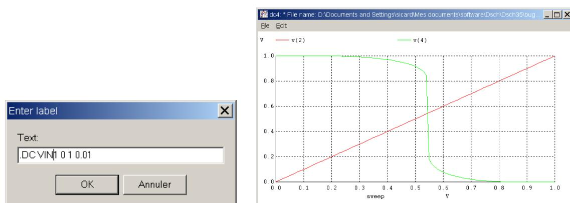
Figure 10: the transfer characteristics of the inverter using DC simulation (spice/spiceinvdc.sch)
